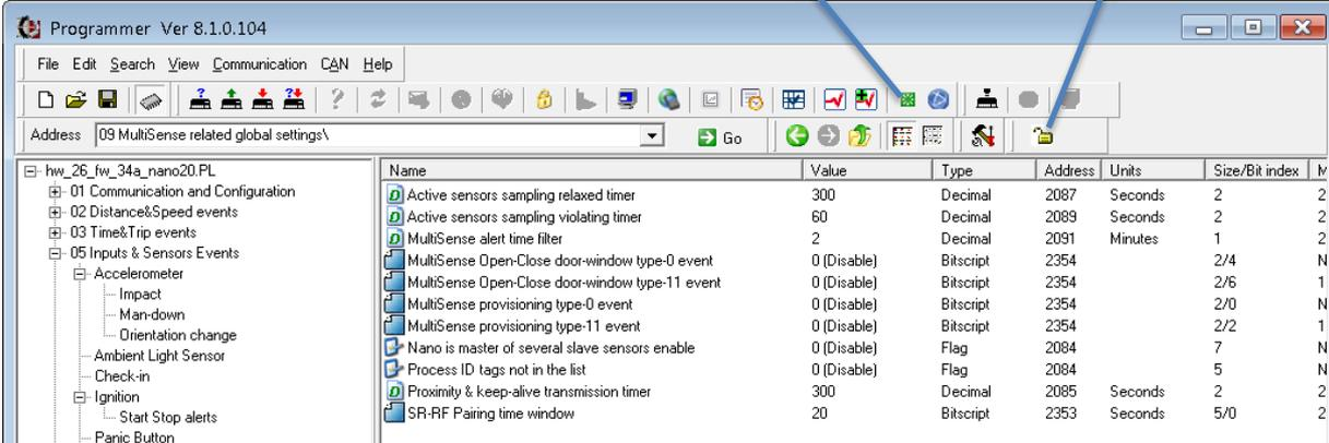
The screenshot shows the Programmer software interface (Ver 8.1.0.104) displaying MultiSense parameters. The interface includes a menu bar (File, Edit, Search, View, Communication, CAN, Help), a toolbar, and a main window with a tree view on the left and a parameter table on the right. The tree view shows the following structure:
